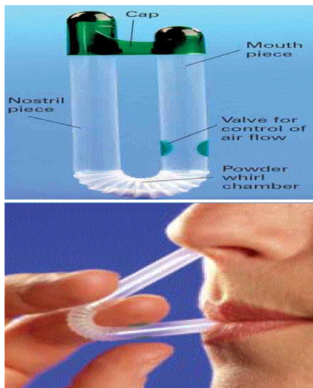
Figure 7: Schematic presentation of DirectHaler™ Nasal device and its way of usage
