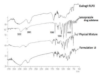
**Figure 4:** FTIR spectrograms of Eudragit RLPO (A), Lansoprazole drug substance (B), Physical mixture of ERLPO-LSP(C), lyophilized Formulation L3 (D).
