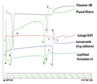
**Figure 2:** DSC thermograms of Poloxamer 188 (A), Physical mixture of LSP/ERLPO (B), Eudragit RLPO (C), Lansoprazole drug substance (D), Lyophilized Formulation L3 (E)
