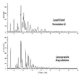
**Figure 3:** PXRD spectra of lansoprazole (A), Lyophilized Formulation L3, (B)
