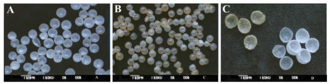
**Figure 1:** SEM image of indomethacin microballoons with (A) coat: core ratio of 2:1, (B) coat: core ratio of 1:3 and (C) inside view.
