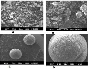
**Figure 3:** Scanning electron photomicrographs of the Co-processed (A), Physical mixture (B), Formulation(C) and Pellet surface
