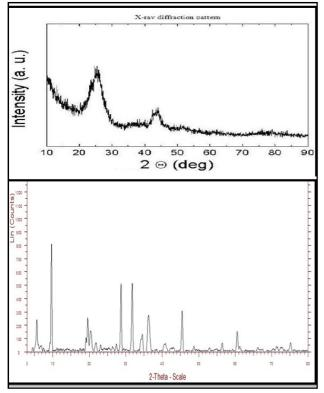
**Figure 2:** X-ray powder diffractions of silicon dioxide (A) and co-processed calcium stearate – silicon dioxide (B).
