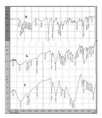
**Figure 4:** FTIR spectra of a) Pure Irbesartan b) physical mixture c) Formulation
