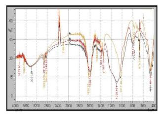
**Figure 1:** FTIR spectra of A) calcium stearate B) silicon dioxide C) co-processed calcium stearate – silicon dioxide.
