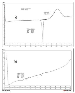
**Figure 5:** DSC thermograms of Pure irbesartan (a) and Pellet formulation (b).
