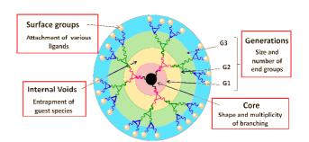
**Figure 2:** Schematic representation if generation of two dendrimres
