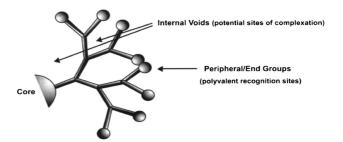
**Figure1:** Three main parts of a dendrimer: the core, end-groups, and subunits linking the two molecules.
