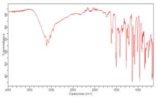
Figure 1: FTIR spectrum of pure Fluconazole
