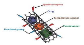
**Figure 2:** Schematic highlighting- the versatile functionalization possibilities of carbon nanotubes.
